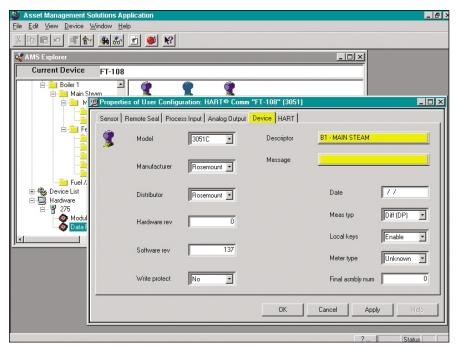
The Model 275 HART\* Communicator Interface lets you update your AMS database to maintain up-to-date records of field device configurations.
